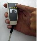
Push the ON/OFF button at the control unit to start operation. All LEDs of the control unit will light. Simultaneously, the blow-out mode will be triggered for approximately 5 seconds. Air will be blown through the electrodes with increased power in order to remove any residual moisture. Starting at the highest pressure level, the LEDs will turn off one after another, until all but the one for the lowest pressure level
